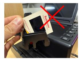
**5. Insert the tray** in the lowest groove on the left side of the machine until it gently touches the transport arm.
