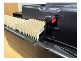
**6.** Check the Framing: Press the right arrow button, then press OK to select Framing. The transport arm will grab the first slide and insert it into the machine.
